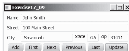
FIGURE 17.20 The application can store, retrieve, and update addresses from a file. Source: Copyright © 1995–2016 Oracle and/or its affiliates. All rights reserved. Used with permission.
