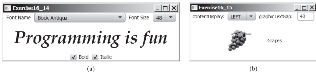
FIGURE 16.42 You can dynamically set the font for the message. (b) You can set the alignment and text-position properties of a label dynamically. Source: Copyright © 1995–2016 Oracle and/or its affiliates. All rights reserved. Used with permission.
