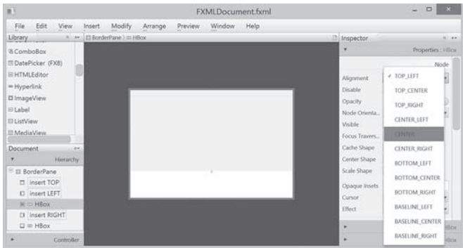
FIGURE 31.42 A BorderPane is dropped to the UI and an HBox is placed at the bottom of the BorderPane.
