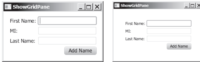
FIGURE 14.19 The GridPane places the nodes in a grid with a specified column and row indices.
