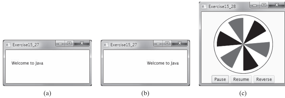
FIGURE 15.35 (a and b) A text is moving from left to right circularly. (c) The program simulates a fan running.
